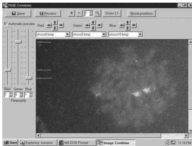
Figure 19. User interface for color composite fusion, with precise recentering and color balance controls, shown with arrows, provide user with real time insight into color composite generation... (preprocessing and monochrome compositions not shown)
