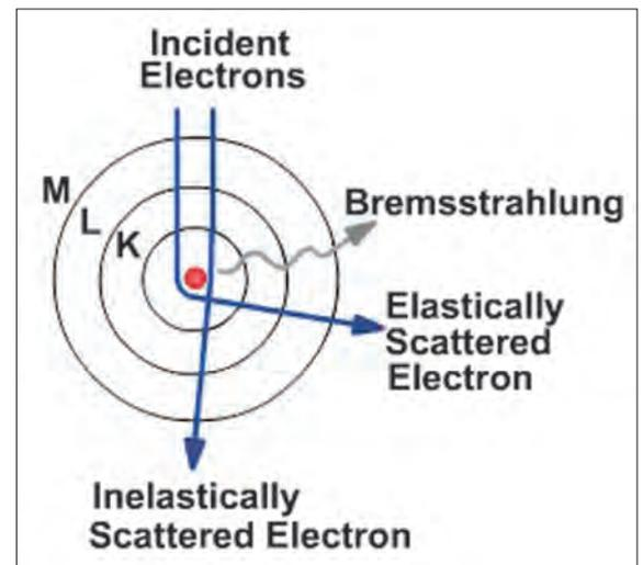
Figure 3. Scheme of X radiation or „braking radiation" (20)
