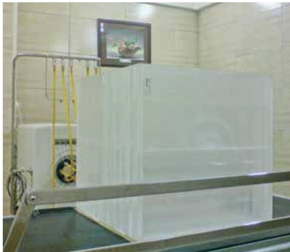
Figure 3. In phantom measurement set-up showing the GZP6 afterloading unit and the perspex phantom
