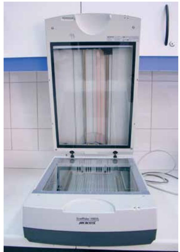
Figure 2. The Microtek 1000XL scanner used in this study for RCF readings
