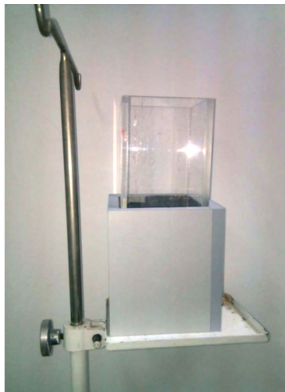
Figure 1. The shield used for PRRT application (Lead & Plexyglas)
