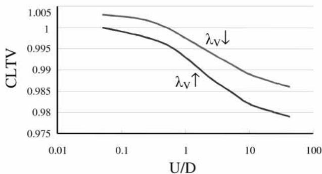
**Figure 6.** Results of CLTV simulation. (U - contributions of convective and D diffusive radon entries to indoor radon concentration, ↑ - case air exchange rate long-term increasing, λ<sub>v</sub>↓ - case air exchange rate long-term increasing decreasing)
