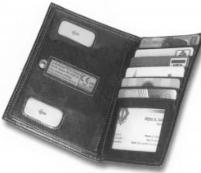
**Figure 1.** Wallet-like ECG recorder
