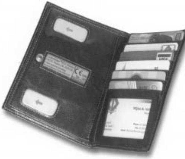
**Figure 1.** Wallet-like ECG recorder
