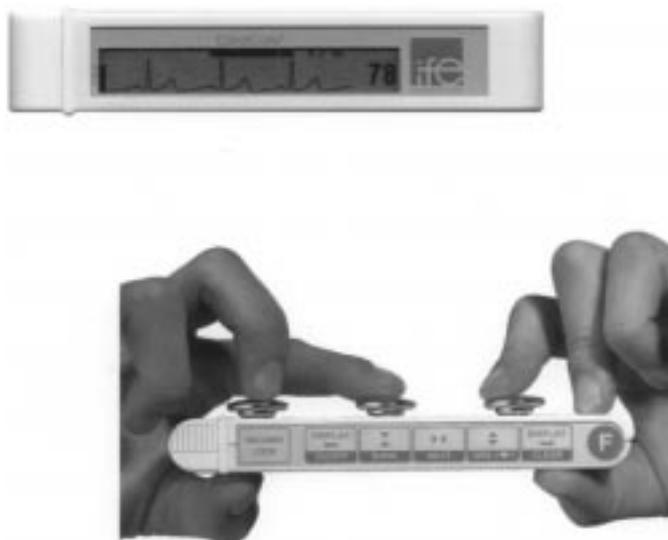
**Figure 2.** Small Tele-ECG monitoring device with metal contacts (Company IFE, Germany)
