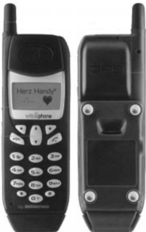
Figure 4. New generation cellular phone with ECG recorder embedded (Company Vitaphone, Germany)
